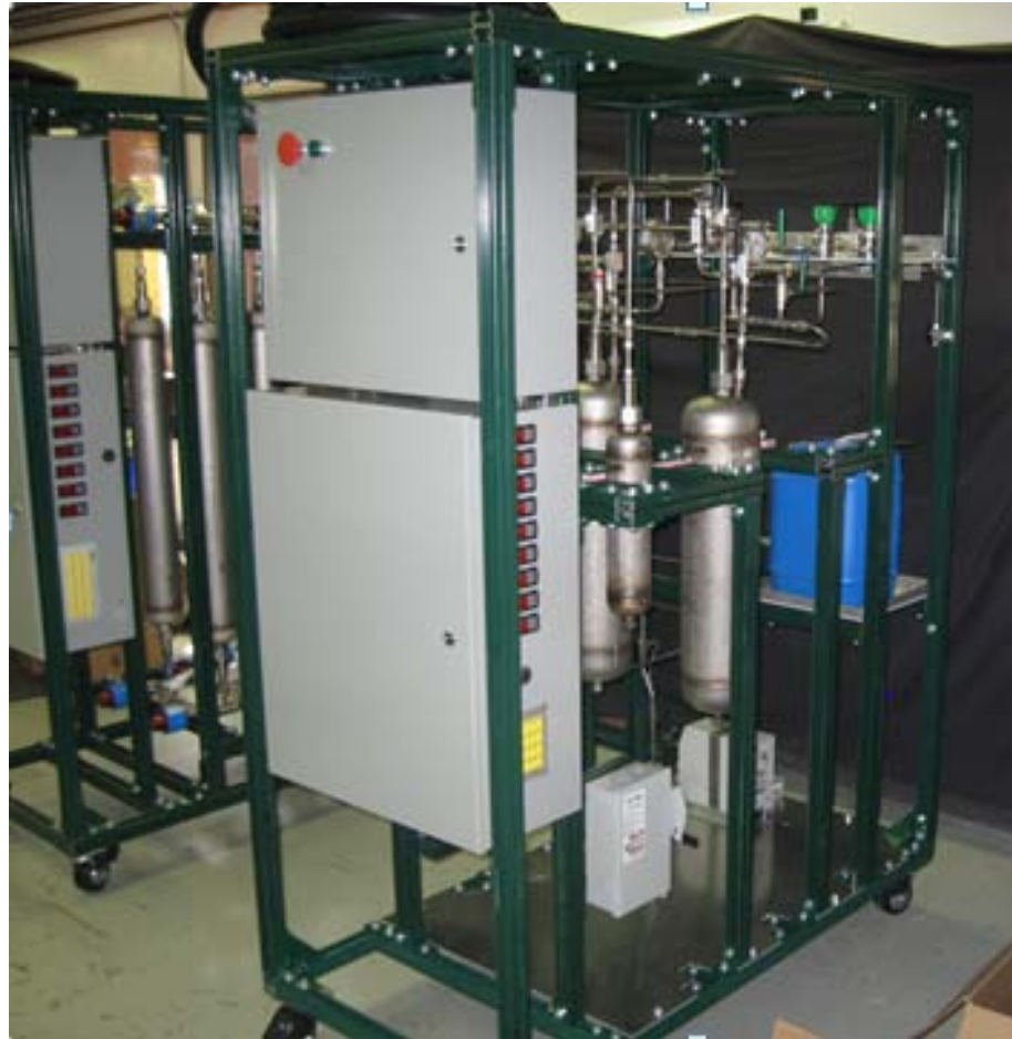
Skid #1 - Synthesis gas pre-treatment skid
